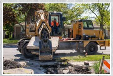
clearance like a conventional excavator's knuckle boom, the XL 4100 V could reach under tree limbs and signs without damaging them. Load-sensing controls automatically eliminate the need for work mode guesswork, saving fuel and emissions.
