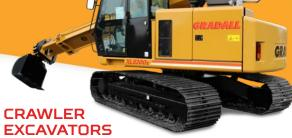
Maneuver on rocks, dirt and sand with Series V Gradall excavators mounted on long, stable crawler undercarriages. Triple grouser excavator pads enhance tracking capability, traveling at speeds up to 3.4 mph. Tracks are powered with dual-range, high-torque piston motors for efficient, reliable carrier travel. Unlike conventional excavators, the telescoping boom delivers consistent, productive cycle times, even on low-overhead jobs.
