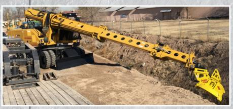
positioned, the mulcher can dispose of trees up to eight inches in diameter. Full boom tilting action also allows the operator to position the mower at an angle that matches the slope of the banks, removing vegetation but leaving roots
