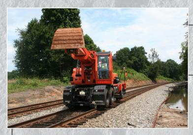
Calvin can reposition the machine from the upper-structure cab – moving both forward and backward as needed. To remove
