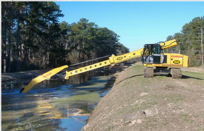
to get the job done.” ❖ A new Telestick design is much more robust with harder material at the pivot points, creating less boom swing when removing buckets full of material. The design is fast and easy to install, hooking onto the bucket adapter. ❖ “That comes in handy when we switch between the Telestick and a
