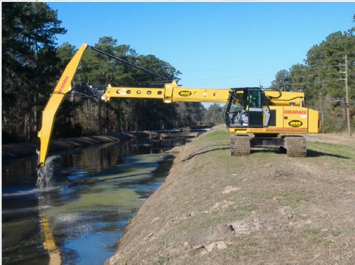
220 degrees to work on the slopes and side of canals. ❖ The XL 5200 III excavator is the largest construction model in the Gradall crawler collection, weighing just over 54,000 pounds. Designed to handle a range of high-productivity jobs, the machine uses load-sensing hydraulics
