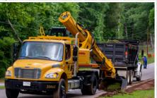
openings to drainage pipes under driveways. Sometimes, this work also involves removing broken pipes and installing new ones. On this job, the operator also manipulated the boom to straighten two mailboxes that had leaned over in time. The compact size of the Discovery Series models makes them ideal for work in municipalities, said Moss,
