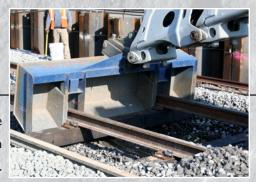
The bucket and the smooth Gradall telescoping movements evenly distribute and smooth ballast much faster than if it was spread by hand. The low working profile of the Gradall also allows it to work in tunnels or under structures. \* "Before we used the Gradall for this type of work, we used manual labor," said Jonathan Barnhart, project manager for J-Track "A team of four men could typically remove and replace 20 ties a day by hand. Using the Gradall and the grapple,
